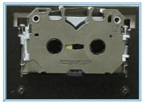
When loading the Ribbons in the Ribbon Compartment, Make sure you remove the cardboard stopper, and place the ribbon in the holder so the "B" side faces out. Take up the slack in the ribbon before installing it into the holder.
